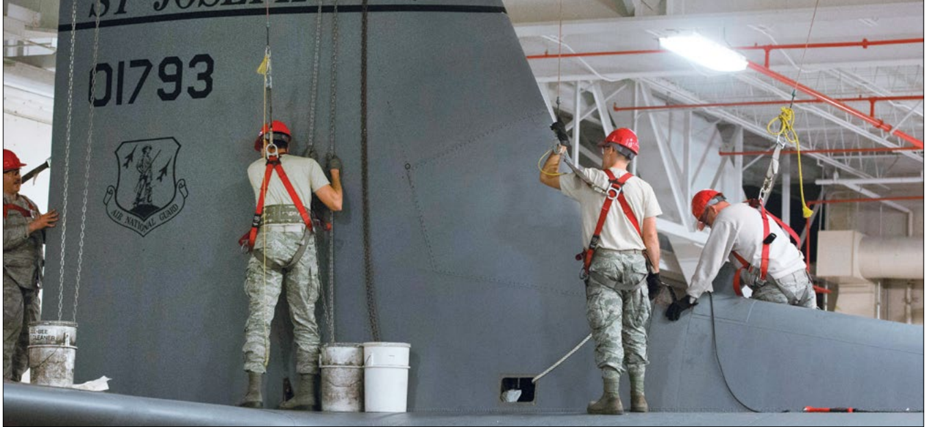
Airmen prepare to remove a vertical stabilizer from a C-130 at Rosecrans ANGB, Mo.
