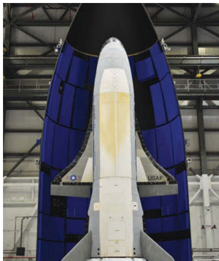
Encapsulated X-37B Orbital Test Vehicle for United States Space Force-7 mission at an undisclosed location May 6.
